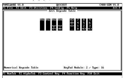
Save the key assignments by pressing the F10 Exit function key.
